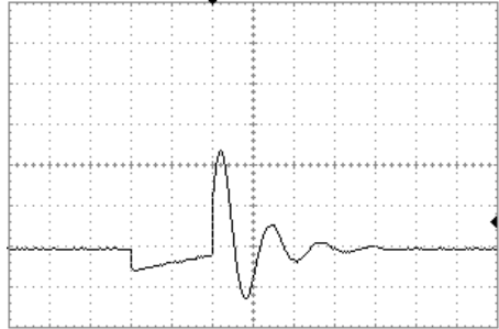
Load L1; S2 – 'Off', load capacity – 33 nF
