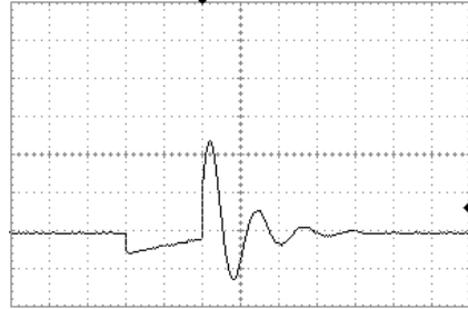
Load L1; S2 – 'Off', load capacity – 33 nF
